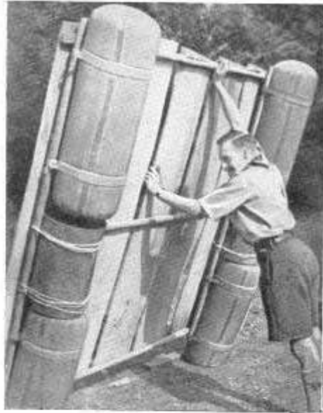
ALTERNATIVE METHOD OF ATTACHING INFLATED BUOYS
