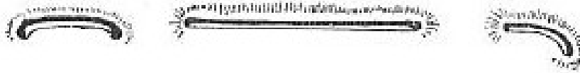
Line of trenches open to enfilade by distant artillery or rifle fire, or to be fired into from the rear.
