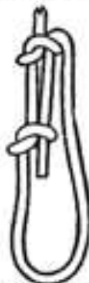
GUY-LINE HITCH can be lengthened or shortened as needed.
