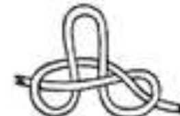
MAN HARNESS KNOT makes a pulling loop in tow-rope.
