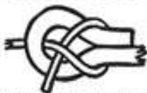
SHEET BEND for joining ropes of equal or unequal thicknesses.
