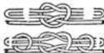
FIREMAN'S CHAIR KNOT has two loops for lowering persons.
